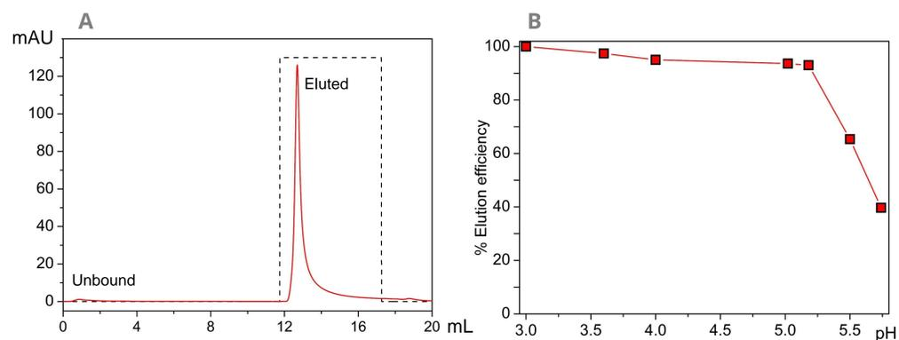
**Figure 5A.** Example trace demonstrating elution of hIgG from Affimer D11 resin using MES (pH 5.2) elution buffer. **5B.** Elution efficiency of Affimer D11 resin across a range of pH values.
