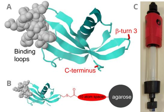
**Figure 1A.** Structure of the Affimer scaffold protein with the two regions containing variable amino acid loops in grey. **1B.** Schematic showing conjugation of Affimer protein to agarose resin. **1C.** Column loaded with affinity resin.
