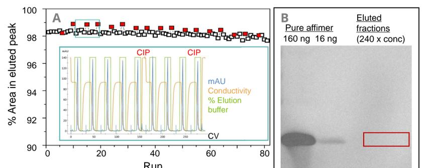
**Figure 4A.** An Affimer D11 column demonstrated high levels of reproducibility over 81 consecutive purification cycles. **Inset:** Example traces for a section of the experiment. **4B.** Example western blot indicating no detectable leaching during elution, pure Affimer protein is included for reference.
