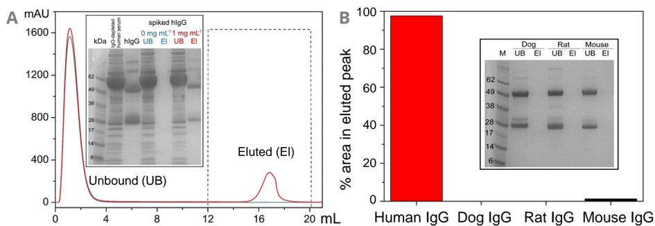
**Figure 2A.** Traces produced upon loading IgG-depleted human serum spiked with known concentrations of hIgG onto Affimer D11 resin. The wash buffer used is PBS (pH 7.4) and elution buffer is glycine, NaCl (pH 3.0). **Inset:** SDS-PAGE (under reducing conditions) confirms specificity of binding and elution. **2B.** % Area of elution peak after injection of 1 mg of pure immunoglobulins.
