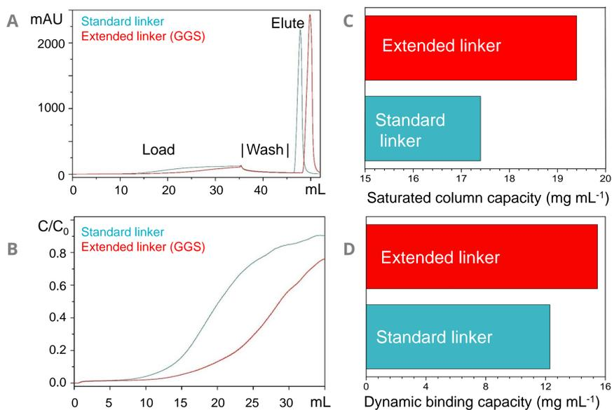
**Figure 3.** Dynamic binding during continual loading of 0.5 mg mL<sup>-1</sup> pure hIgG over Affimer D11 resins with a column residence time of 3 min. **3A.** Full traces showing load, wash and elution phases. **3B.** Normalised breakthrough curves. **3C.** The amount of target protein recovered during elution, normalised to column volume. **3D.** The dynamic binding capacity at 10 % breakthrough, normalised to column volume.
